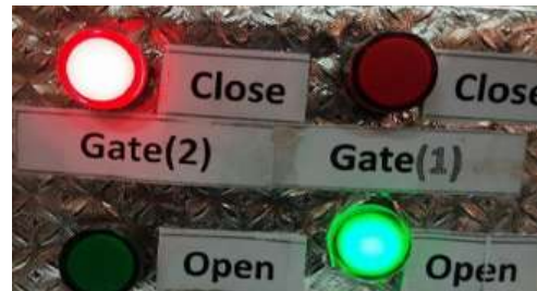
Figure 23: indicator lamps for stage 2.
